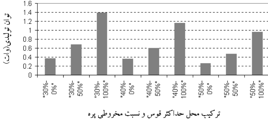
Figure 16: mutual effect of place of maximum arc and conical ratio on output power
