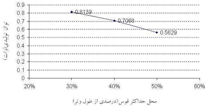
Figure 14: effect of place of maximum arc on output power
